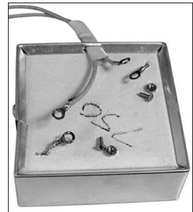
Figure 10 - Lead wires disconnected from element.
